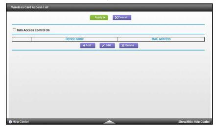
From the Wireless Card Access List screen, click **Add** to display the Wireless Card Access Setup screen. On this screen, you can restrict access to your network to specific devices based on their MAC address.
